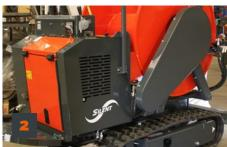
Enabling contractors to undertake jobs at a distance from the jetting machine, these robust units are custom built in a range of configurations to suit the work requirement. The most common caterpillar track systems are especially suited to off-road terrains, such as fields, golf courses, railway embankments and canal or river sides.
