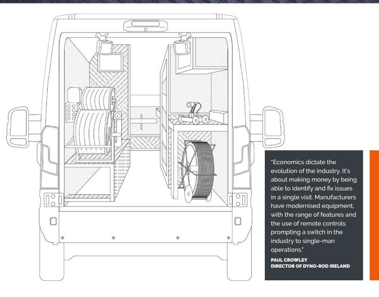
Drainage vehicles have evolved in recent years, with multipurpose vans that can be operated by a single person becoming much more the norm. These types of made-to-measure vehicles are designed and equipped to carry out multiple tasks in a single visit.
